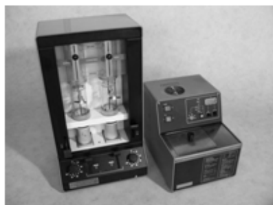
Rys.3. Aparat 1045 SOXTEC SYSTEM HT-2 firmy Foss (Dania)
